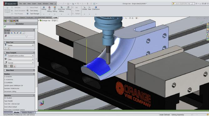
Finish paths follow part faces to create the final part shape. HSMWorks generates surface finish using machining technologies that incorporate smooth/tangent lead in/out moves to keep the tool moving in a smooth motion, helping to reduce machine wear and tool marks.
